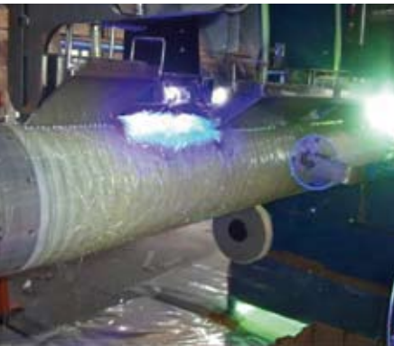
Figure 2 Production of a fiberglass tube with polymerization induced by UV rays, using dual curing formulations developed by CimtecLab.
