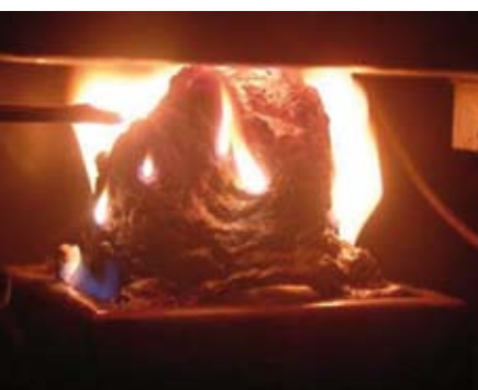
Figure 1 Intumescent behaviour during a cone calorimeter test.
